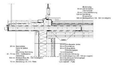
Figure 3. Example: Mitigation of thermal energy dissipation in cantilevered timber structures [6]
