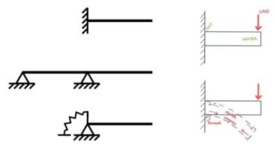
Figure 1. Cantilever beam [5]
