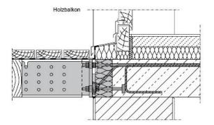
Figure 2. Example: Mitigation of thermal energy dissipation in cantilevered timber structures [6]
