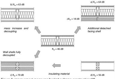
Figure 6: improvement measures for timber frame constructions[2]
