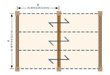
Figure 1: Typical post-beam-panel system grids
