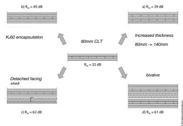
Figure 6: improvement measures for solid timber constructions [2]
