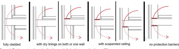
Figure 4: Basic construction rules for the need of elastic separation layers [3]
