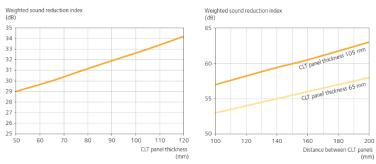
Figure 3: Sound insulation improvement by CLT panel thickness compared to improvement by distance of two CLT panels [2]
